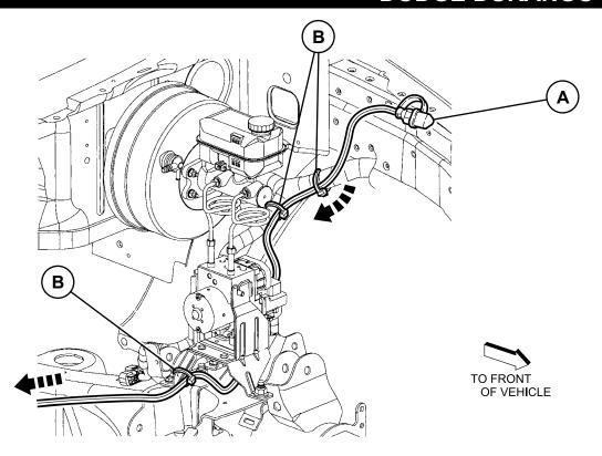
Open the hood. Position cordset plug as shown. Route cordset down into the left (driver's side) of the engine compartment. Keep away from any sharp edges, heat sources, or moving parts. Secure cordset as shown with supplied tie straps.
