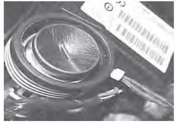
F. Re-install the SKIM/SKREEM module to the ignition cylinder and secure with the screw. Make sure to plug the connector back into the SKIM/SKREEM.
