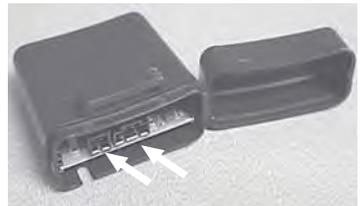
H. Close the flap on the SKIM/SKREEM Interface and secure with a supplied tie wrap.
