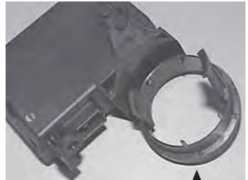
Transceiver Antenna Coil
