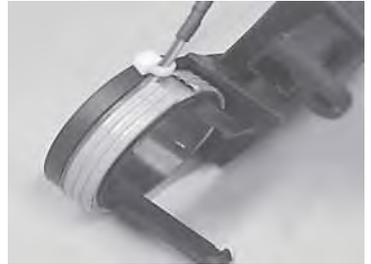
E. Using a supplied wire tie, secure the antenna coil as shown.
