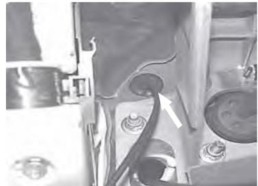
J. For gas engines route the Blue/Green wire to the top of the engine at the coil connection point as shown.
