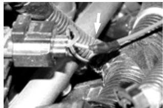
I. Route the Green and Yellow wires to the relay junction box on the driver side of the engine compartment. Remove the horn relay as shown in the diagram. Slide the supplied Green wire relay terminal connector over terminal 85 (pin #1) of the relay as shown in the diagram.
