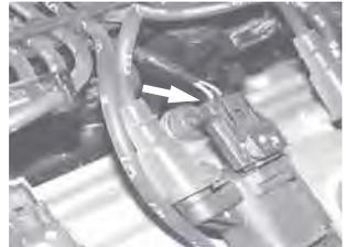
J. Route the Dk Green wire to the relay junction box on the passenger side of the engine compartment. Remove the horn relay as shown in the diagram. Slide the supplied relay terminal connector over terminal 85 of the relay as shown in the diagram. Re-insert the relay into place. Route the wiring from the relay connector out of the junction box and connect to the Dk Green wire using the supplied butt connector.
