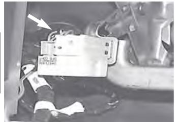
F. Locate the White/Brown wire in pin #1 of the 10-way connector, found at the headlight switch. Center-splice the harness White/Brown wire into this wire, following the center-splice procedure on page 7.
