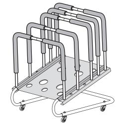
Insert dividers into the holes along sides of pan. Dividers should fit securely into mounting holes.
