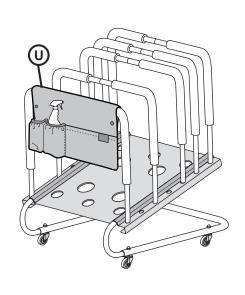
Wrap top of tool caddy around top of a door cart divider and secure with hook and loop fastener. Store tools, hardware and cleaner bottles.
