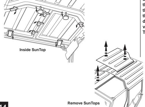
Release the levers that secure the SunTops to the windshield. Release the knobs that secure the SunTops to the rear deck. Release the Levers. Remove the SunTops from the vehicle.
