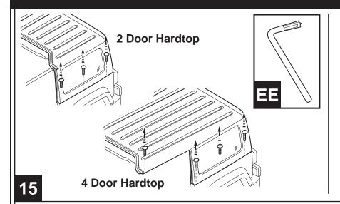
Use the T40 Torx Wrench to remove the six (6) Torx Bolts that secure the 2 Door Hardtop or the eight (8) Torx Bolts that secure the 4 Door Hardtop.
