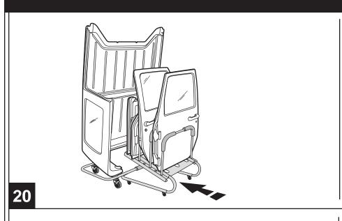
Roll door cart into top cart and load with doors. Center the cart in the top.
