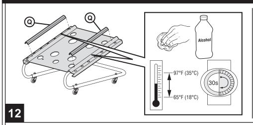
Clean the top of the mounting ridges with alcohol. Place the rubber strips on the top of the mounting ridges, over the truss head screws and center. Peel the backing a little at a time and press firmly into place. Apply uniform pressure for thirty (30) seconds.
