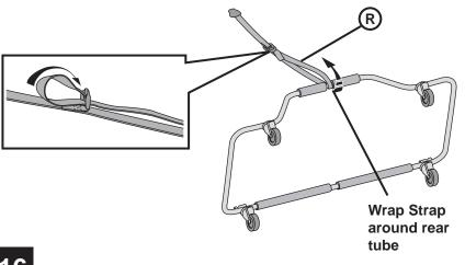
Orient the strap with the buckle facing the rear of the top cart. Wrap the straight end of the strap around the rear tube in the space between the two foam sleeves. Pull it toward the buckle in the middle of the strap without twisting.
