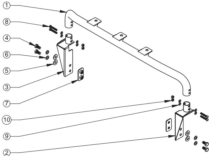
1. Locate the two frame mounting holes behind the bumper on the left side of the vehicle. Slide the Nut Plate behind the two holes. Use the M12 Hex Bolts, M12 Lock Washers, and M12 Flat Washers to secure the Left Side Bracket to the frame as shown. Do not tighten the bolts at this time. Repeat for right side.
