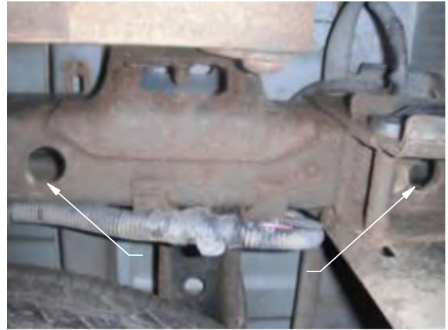
2 Remove (6) M12-1.75 x 55mm bolts attaching the cargo box to the frame using a 18mm socket and extension. Save for use later.
