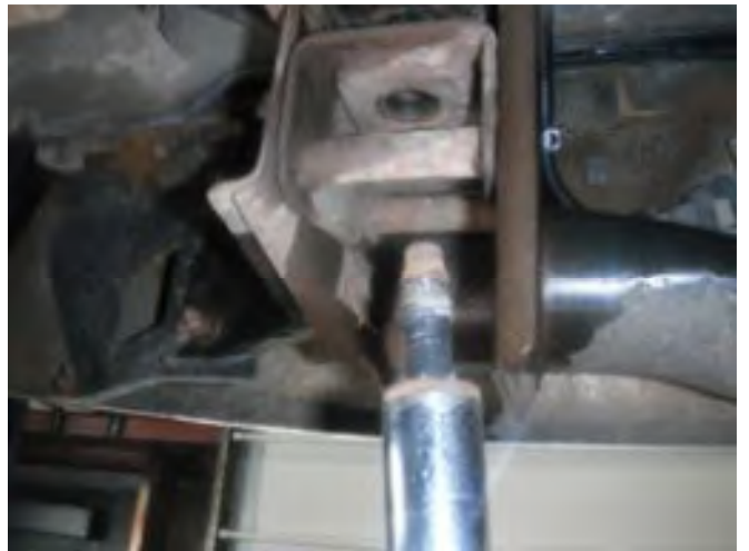
12 Remove (2) M14 bolts from lower bumper mounting bracket using a 21mm socket. Save for later use.
