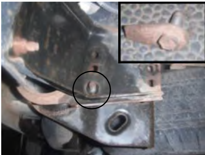
9 Remove (2) flag bolts from bumper mount (1) per side. Save for later use.
