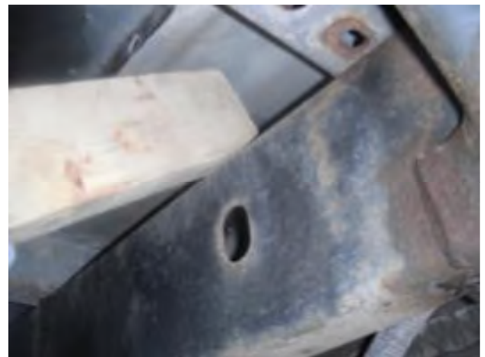
4 Place block between frame and cargo box, lower cargo box onto blocking.
