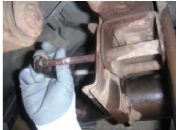
6 Remove (2) bolt tabs, (1) per side and discard. SUPPORT BUMPER DURING BUMPER MOUNT REMOVAL.
