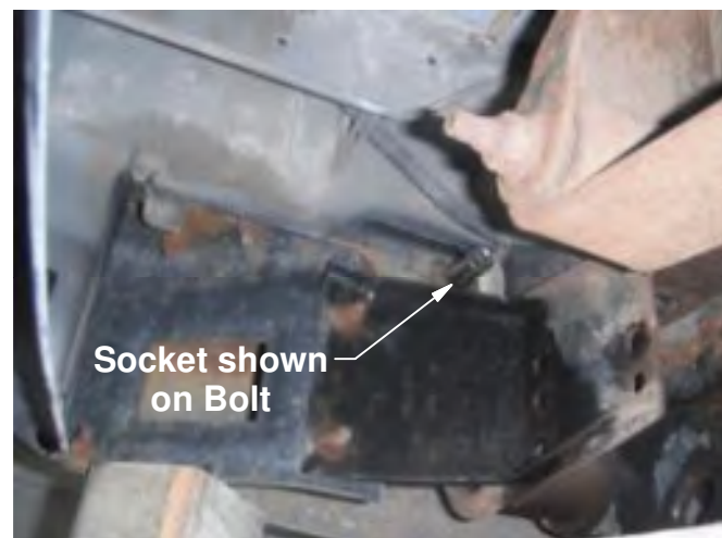
11 Remove (2) remaining bolts from bumper using a 15mm socket. Save for later use.
