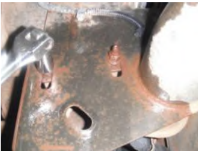
5 Remove (4) M10 flange nuts, (2) per side, with a 15mm socket and discard.
