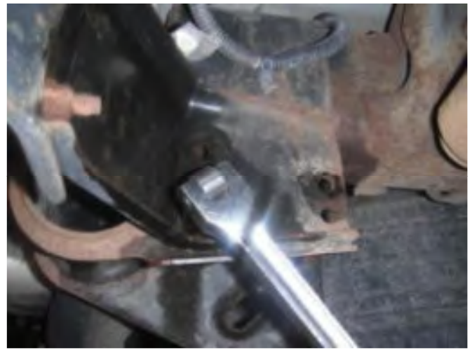
8 Remove (2) M10 flange nuts from the bumper mounting arms using a 15mm socket. Save for later use.
