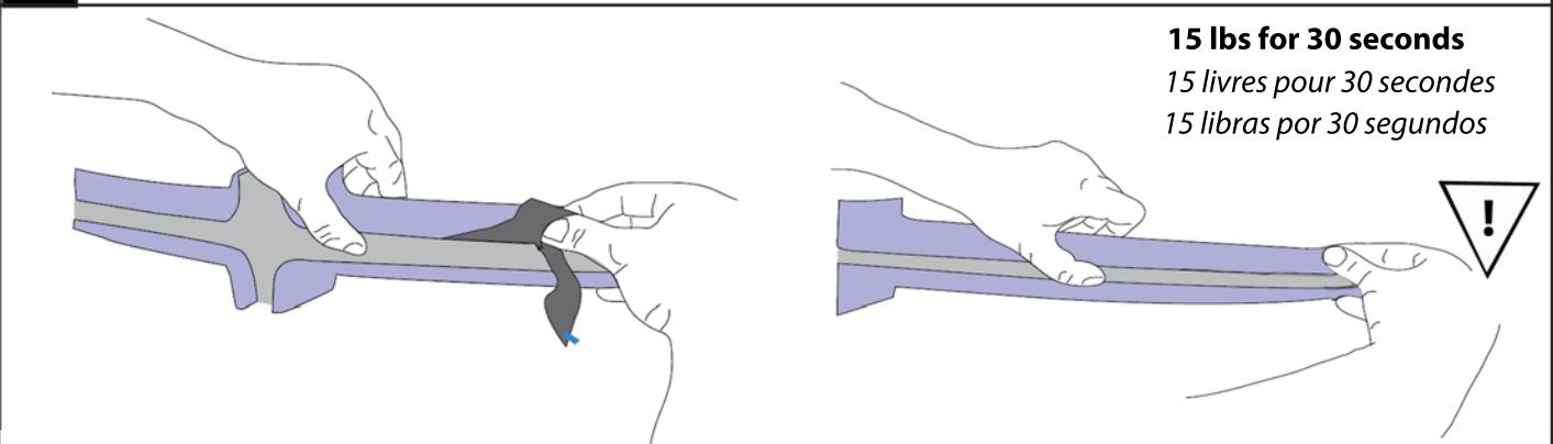
**Continue installing the appliquéd to the grille by slowly pulling the liner towards the end and applying firm even pressure on the top of the appliquéd in the same direction. Apply extra pressure to the end to ensure full adhesion to the grill.**
