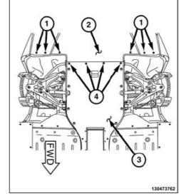
4. Remove the four fasteners (4) connecting the center belly pan (3) to the rear belly pan (2)
