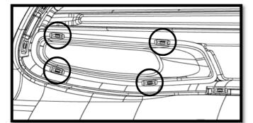
8. Place Passenger Side Carbon Fiber Inlet Bezel (A) and secure it in place using 4 of the provided rectangular push pins (C).
