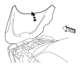
6. With the help of an assistant, remove the fascia by untucking the sides from the wheelhouse and unplugging the front side marker lamps. Place fascia on protected surface.
