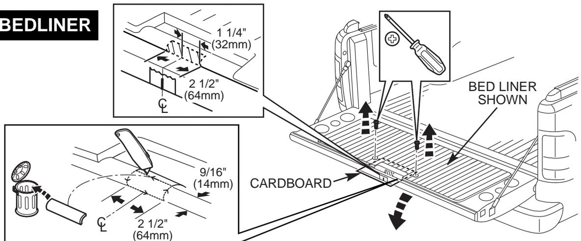
Remove 2 screws in tailgate cover to allow cardboard to be inserted to protect painted surface. **Only** molded bedliner cover needs to be modified (remove 1/2 of the bumped surface). **DO NOT** modify the plastic spoiler cover - the footman loop will attach directly to it. (Refer to step 18A). Remove and discard cardboard.
