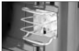
Mounts directly to body behind taillamp
