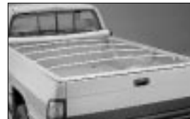
Clamps to side rail, includes bows
