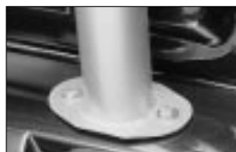
Mounting plate is welded to leg
