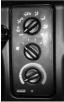
Air Conditioning controls (shown on Truck)
