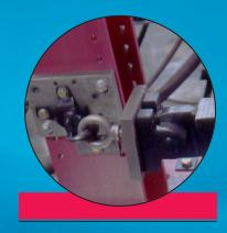
Before they can carry the Mopar name, all Hitch Receivers undergo a series of rigorous tests to meet tough DaimlerChrysler standards for safety and durability. Included in these tests is a weight-carrying fatigue test in which 150,000 repetitions of vertical and horizontal stress are applied to the receiver. This is designed to simulate heavy-duty trailer use throughout the lifetime of the tow vehicle and hitch.
