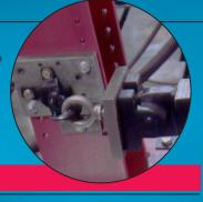
Before they can carry the Mopar name, all Hitch Receivers undergo a series of rigorous tests to meet tough DaimlerChrysler standards for safety and durability. Included in these tests is a weight-carrying fatigue test in which 150,000 repetitions of vertical and horizontal stress are applied to the receiver. This is designed to simulate heavy-duty trailer use throughout the lifetime of the tow vehicle and hitch.
