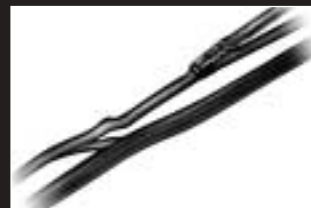
BENT AND/OR CRACKED ARM AND/OR BLADE
