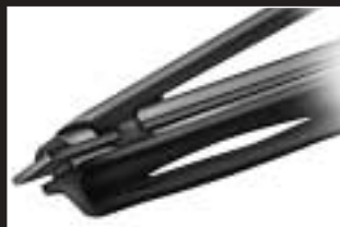
TORN RUBBER PULLED AWAY FROM BLADE (MAKES A SLAPPING NOISE)
