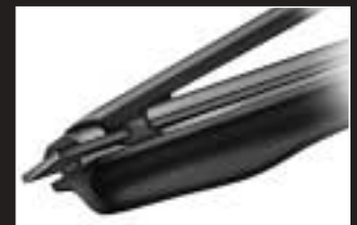
RUBBER LOST FLEXIBILITY (CAN'T FLIP OVER)
